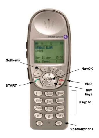
Figure 5.73: Navigation keys on Alcatel-Lucent IP Touch 310/610 WLAN Handsets
