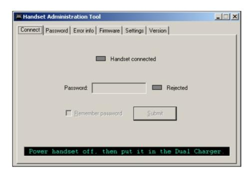
Insert the handset into the Dual Charger and enter the password.
