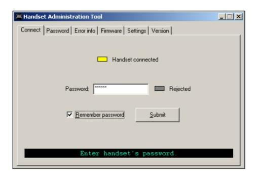
When the handset is inserted for the first time, the password must be entered. If you check the **Remember password** box, the password is retained as the default password for all handsets.
