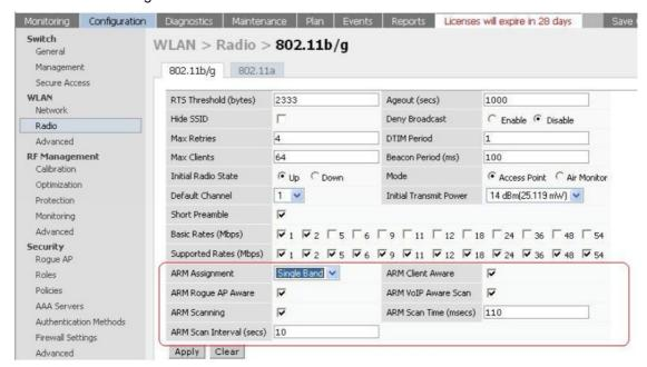
Set the ARM assignment to Single Band to force the APs to select an 802.11b/g channel. Select the ARM Rogue AP aware to enable the AP t detect rogues, ARM scanning has to be enabled to allow the APs to scan the channel and find a cleaner channel. If ARM assignment is set, the AP will move to a cleaner channel based on its preset criteria.
